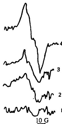
Fig. 7. ESR spectra of samples of MCC before (1) and after micronization for 30 min at 20 (2), 40 (3), and 60 g (4).
